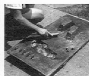
Removing impurities after cast is opened
