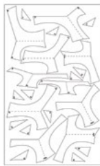
Cut Sheets Cut sheets are generated to produce the jigs and molds from corrugated cardboard.
