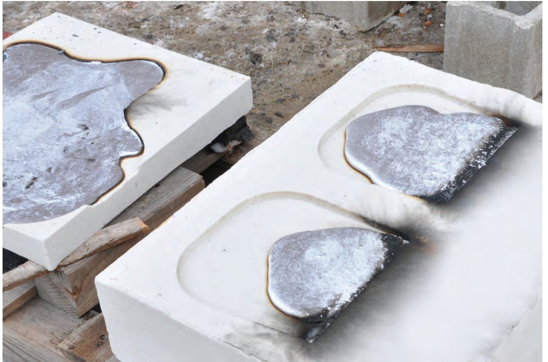
New metal parts in custom sand molds
