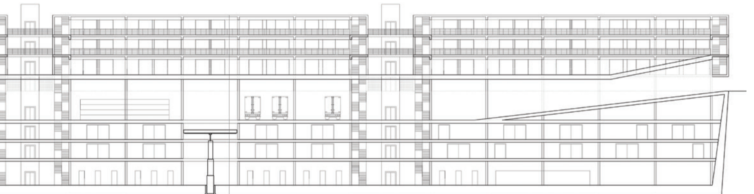
The Long Section showcases the ramps that navigate the elevation change necessitated by the storage facility below. Another portion of a housing structure that has been cut to reveal a double height multi-purpose space that can be adapted to meet the programmatic needs of those living in the housing complex.
