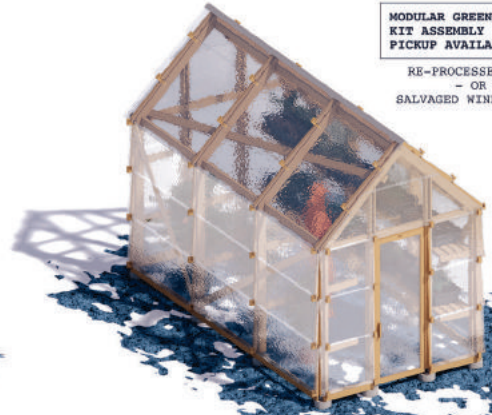
WOOD DOOR FRAME W/ RECYCLED GLASS PANE INSERT SCRAP ALUMINUM RIDGE FLASHING RE-PROCESSED 2" X 6" LONGITUDINAL BEAMS + FURLINS
