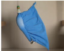
Air pressure: 10 psi Time: 2>3 seconds Transformation: - subtle bending movement - one-area inflation
