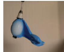
Air pressure: 10 psi Time: 1>2 seconds Transformation: -subtle one-direction flip (fin area) -unified inflation
