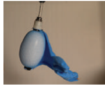
Air pressure: 14 psi Time: 2>3 seconds Transformation: - noticeable one-direction flip (fin area) - subtle elongation
