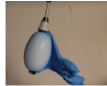
Air pressure: 16 psi Time: 3>4 seconds Transformation: - noticeable one-direction flip (fin area) - noticeable elongation
