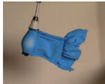
Air pressure: 5 psi Time: 1 second Transformation: unified inflation
