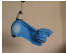
Air pressure: 10 psi Time: 1 second Transformation: -subtle one-direction flip (fin area) -unified inflation
