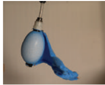
Air pressure: 12 psi Time: 2>3 seconds Transformation: - noticeable one-direction flip (fin area) - unified inflation
