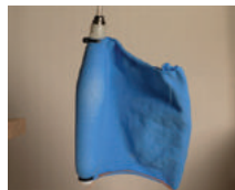
Air pressure: 10 psi Time: 2>3 seconds Transformation: - subtle one-direction flip (fin area) - subtle unified inflation
