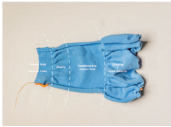
Tubular knit with transitional area and one-side fin
