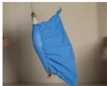
Air pressure: 5 psi Time: <1 second Transformation: minor inflation
