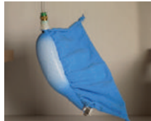
Air pressure: 14 psi Time: 3>4 seconds Transformation: - noticeable elongation - unified inflation
