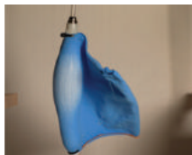
Air pressure: 12 psi Time: 2>3 seconds Transformation: - subtle one-direction flip (fin area) - unified inflation
