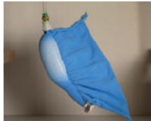
Air pressure: 12 psi Time: 2>3 seconds Transformation: - noticeable elongation - noticeable bending movement
