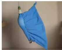
Air pressure: 8 psi Time: 1>2 seconds Transformation: minor inflation
