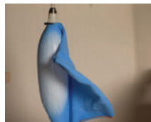
Air pressure: 16 psi Time: 2>3 seconds Transformation: - subtle one-direction flip (fin area) - subtle elongation - unified inflation
