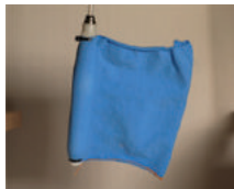
Air pressure: 2 psi Time: <1 second Transformation: minor inflation
